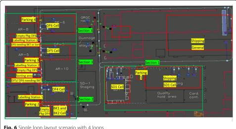
Fig. 6 Single loop layout scenario with 4 loops
